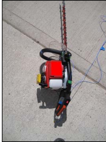
Figure 6 Rear handle rotated through 90°
