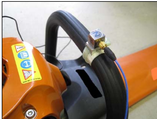
Figure 4 Aluminium block positioned using the cable tie system
